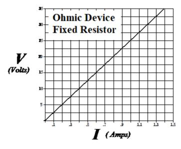
Even in a non-Ohmic Device V=IxR at any point in the graph.
