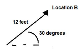
Here the displacement is 12 feet at an angle of 30 degree from the original position A. The Line is called a **vector.** A vector has magnitude (12 feet here) and direction (30 degrees). If you move again, we would represent that move with a second vector added to the end of the first. As shown below.
