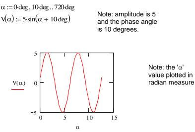
In electronics it is often necessary to plot the voltage versus degree or rotation. For this to occur in MathCAD, we must define an angular function. Then we plot this function on our horizontal axis. This will override the default of MathCAD to plot in radians. For example:
