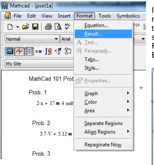
In the file the answers are given to way to many decimal points. To force the display to something reasonable for electronics, say 3 decimal points, click on Format> Results and then set the screen as shown. Be sure to check off the box as shown.
