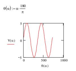
Note: See how the Theta function allows plotting to 720 degrees. Mathematically these are referred to as parametric equations.
