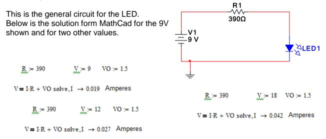
The Mathcad file LEDcirc.mcd will provide the above solution. Note that the solve has had the variable name listed for which we wish to solve. This will work for any equation with multiple values involved. A typical circuit in Basic Electronics is be able to solve the following circuit :
