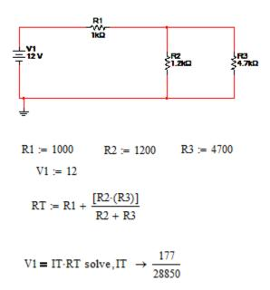
This is file **serpar circuit.msn** on the book CD. The fraction at the end is easily converted to a decimal of 0.0061 Amperes. The solve feature finds an exact solution if possible, and a decimal would be only approximate. Notice that with the MathCad solution the steps are in agreement with the Process described in the paper on **Solving Problems Like A Pro** found in the appendix.
