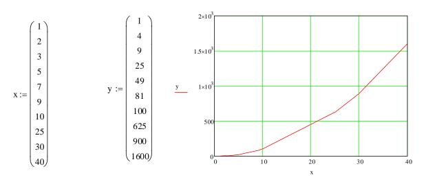
This is a quadratic function. We could quickly confirm this by plotting on log-log paper. The result will be as shown below, and the straight line will confirm a power relationship. (See the appendix on graph shapes.)
