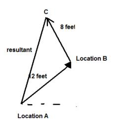
$y=V \sin (\Theta)$  and  $x=V \cos(\Theta)$  Where  $\Theta$  is the angle with the horizontal and V is the length of the vector. For the vector above
