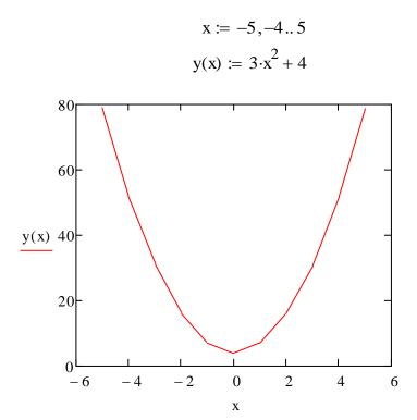
This graph is using the MathCad default values. We can change that by overriding the graph values. Click on the graph to place a black box around the graph as below and change the limits as needed.
