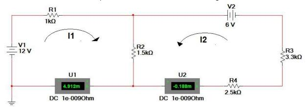
We have assumed two currents as shown from + to – for each battery source. Bsed on this convention then the voltage drop on R1 is -I1 R1, and on R2 it is -(I1+I2) R2. The negative is because for the current to move as shown the right side of R1 would be negative with respect to the left side. The equations then become
