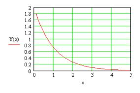
One prominent feature of the  $e^x$  curves is that in a fixed unit of time (the time constant, the Greek letter tau,  $\tau$ ) the curve will drop by 63% in one  $\tau$  and in  $5\tau$  it will drop to nearly level. For your coffee this means it is at room temperature. Knowing the time constant of a system can be useful. This is a constant of the system and does not depend on the high or low
